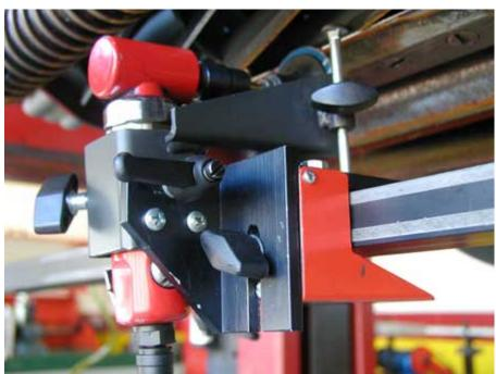
So, this is the finished product, a 5 degree front facer. You are still able to get a degree or two more by increasing the disk pressure, but I usually use a little tougher disk than what comes standard. The setup on the reel is just like the setup on the grinder, touch both ends and adjust from there.
