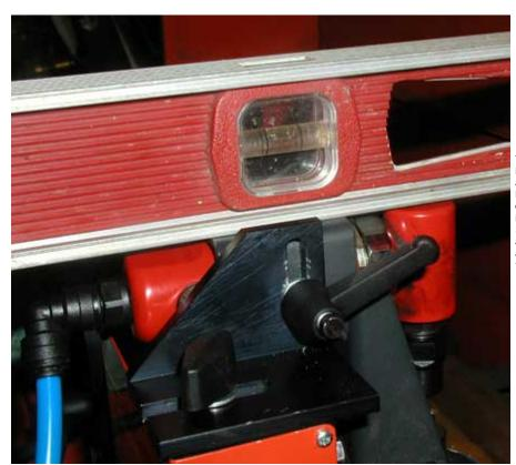
The bar is Zeroed out, the indicator is shown to be accurate. Now I have the RF attached to the front of our beknife grinder, which is an Express Anglemaster 3000. So the bar is level and now I'm checking and adjusting the housing of the RF to level.
